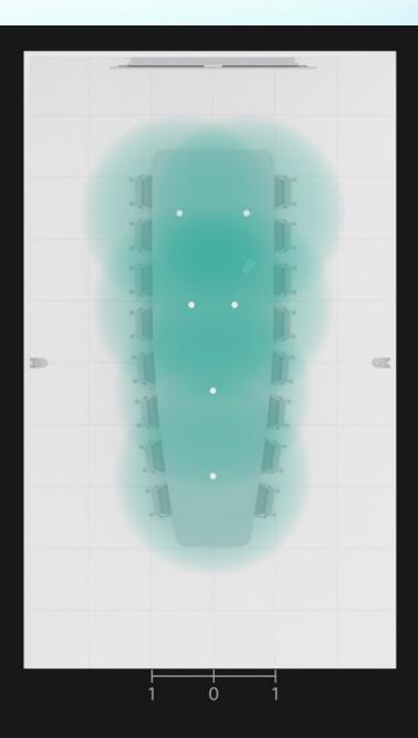
Cisco Table Microphone Pro pickup range per unit (up to 3 m / 10 ft)
