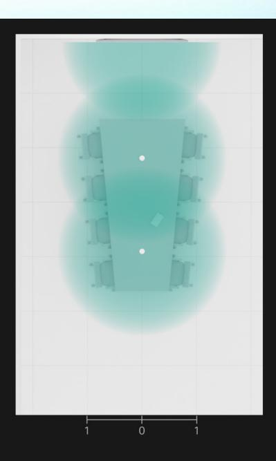
Cisco Table Microphone Pro pickup range per unit (up to 3 m / 10 ft)
