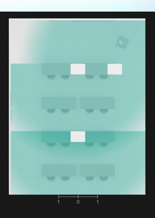
Cisco Ceiling Microphone pickup range per unit (up to 4 m / 13 ft)
